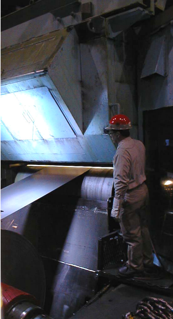
Fig 2: Automated Surface Inspection – Temper Mill Photo Courtesy of Bethlehem Steel
