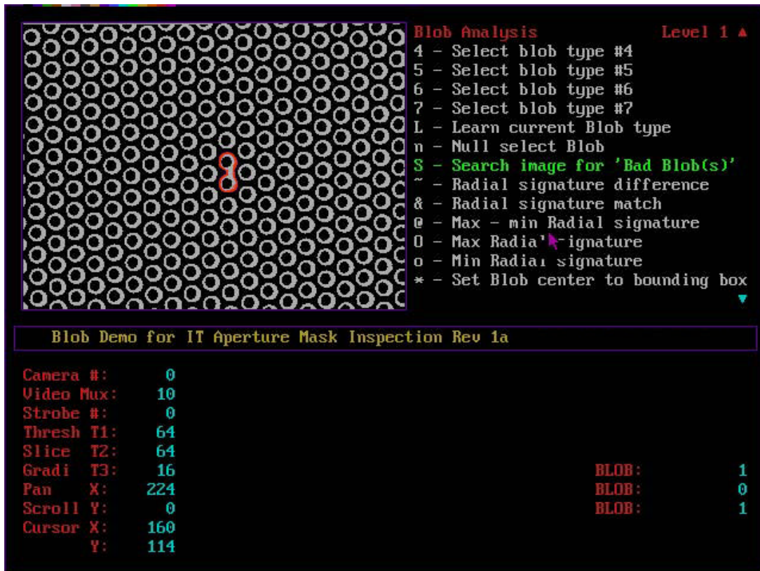
Fig 6: Proprietary algorithm finds minute defects extremely fast using PC based processing techniques. Training of the system can be automated and classifications made based on a number of robust & field proven parameters.
